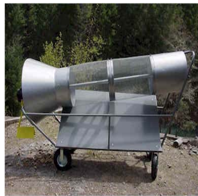
Fig 5: Small to medium-scale harvesters such as this one can be used to harvest hundreds of pounds of worms per day.
